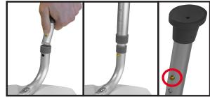
Insert the L-shaped back tubes into the backrest tubes. As you slide in the L-shaped back tube, push the brass button on the backrest tube until the brass button protrudes out of the hole of the L-shaped back tube. Ensure that the brass button "clicks" and locks into position.
